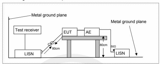
LISN: Line Impedance Stabilization Network
